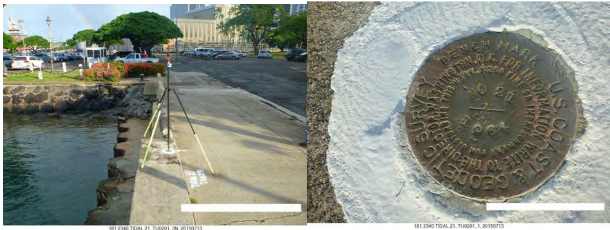
Figure 1. Local Mean Sea Level (LMSL) datum for Oahu is Station 161 2340 TIDAL 21 (PID TU0291) at a height of 2.042 m.
